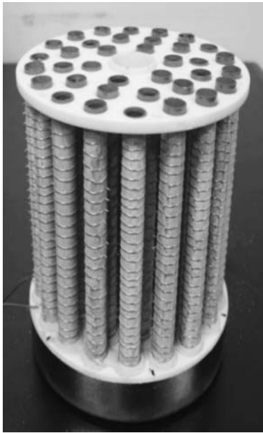
Fig. 3 Bundle of small SOFC tubes for 200 W, operated at \sim 800^\circ\text{C} (Ref 7)
